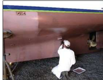
Coppercoat® 4th coat being rolled over 3rd coat.
