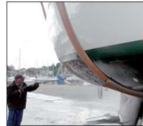
Coppercoat® 4th coat being rolled over 3rd coat.
